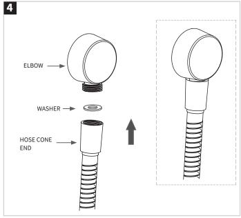
Connect the hose cone end and washer with the elbow.
