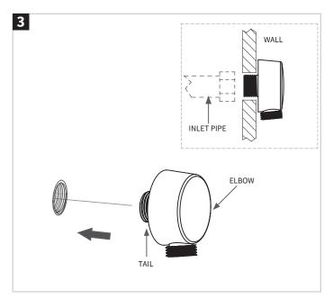
Connect the elbow with the outlet using a suitable thread sealant
