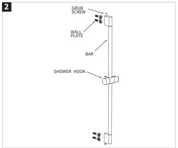
Make sure the shower hook at a suitable position. Fix the bar to the wall plates with grub screws.
