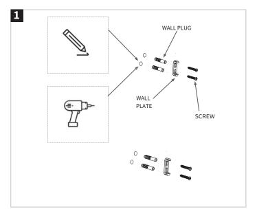
Make sure all is right, mark out the four fixing hole positions on wall. Drill holes. Insert wall plugs. Fix the wall plates onto the wall by screws.
