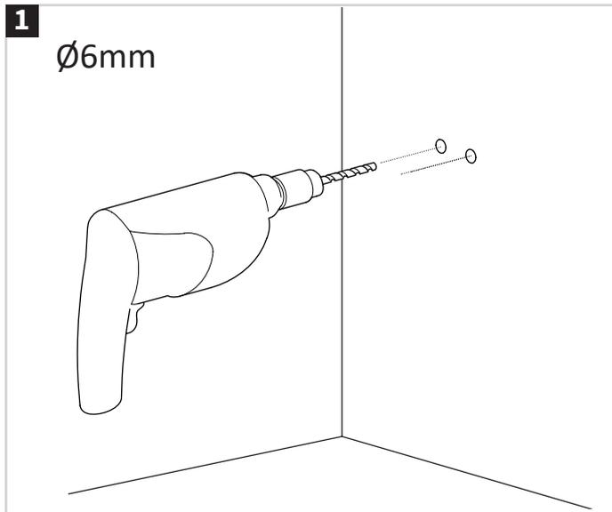
Measure area where accessory will be installed. Use drill to create holes.
