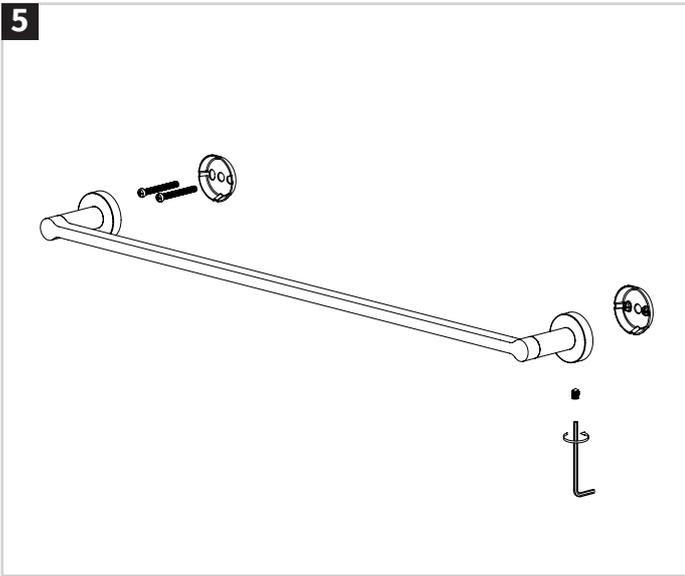
Repeat steps 1-3 for double bracket accessories, ensuring the brackets are level before fixing the accessories in place.
