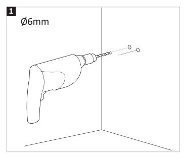
Measure area where accessory will be installed. Use drill to create holes.
