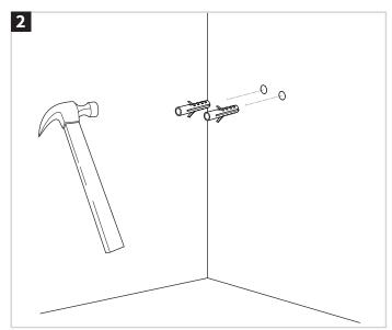
Place rawl plug in hole and use hammer lightly to ensure fully in the wall. Note: The fixing provided are for solid walls. For any other wall type, please use the appropriate fixing.
