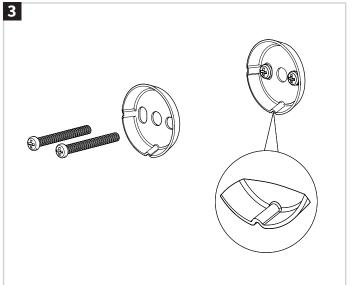
Align base holes with raw plugs in the wall and use a screw driver to secure in place. Ensure that the grub screw notch is positioned facing down.
